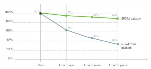
\*Behaviour of a gasket in the event of recurrent compression, e. g. opening and closing of the window.
